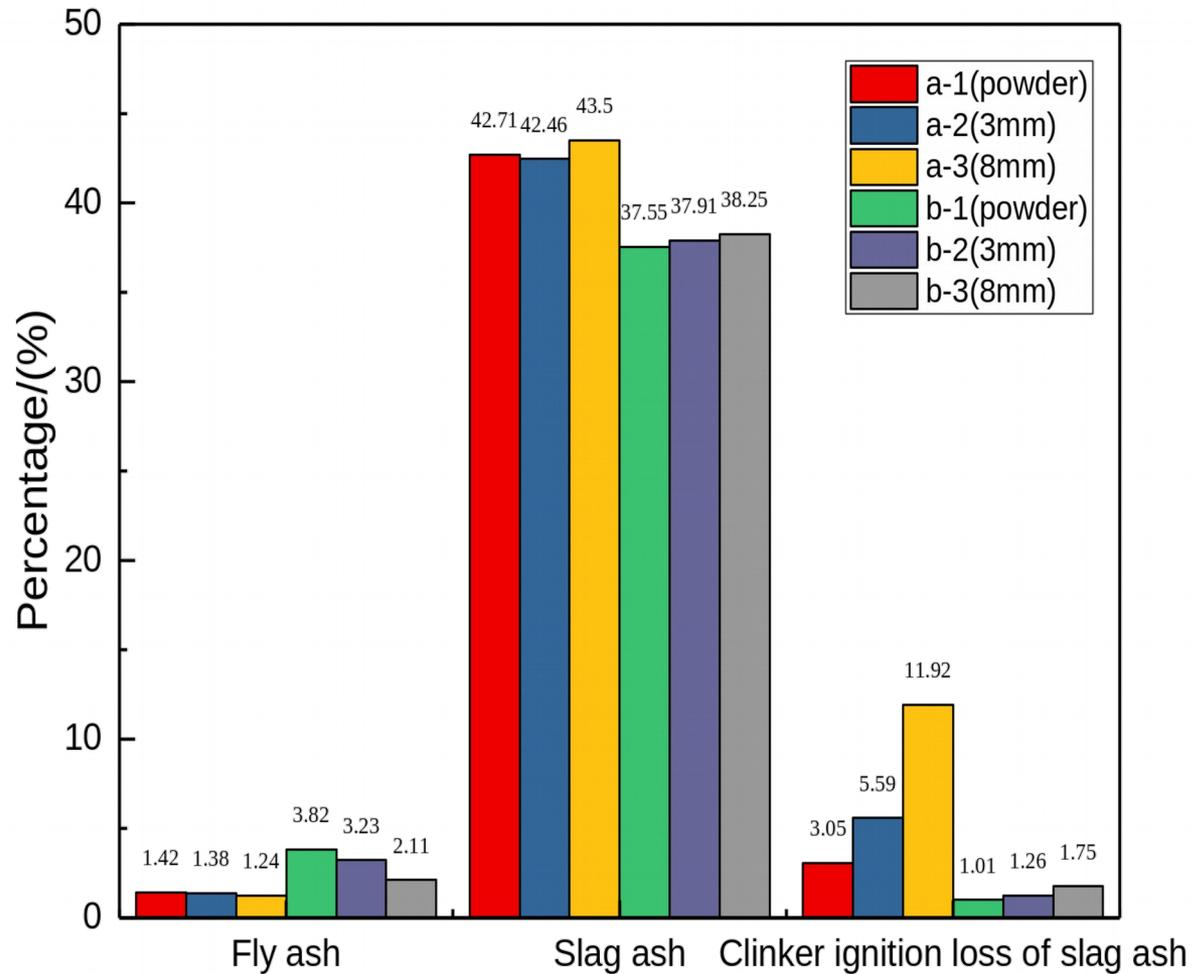
**Ash characteristics at different experimental conditions**
